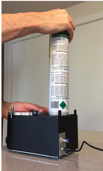
(Fig-2) Install gas bottle
