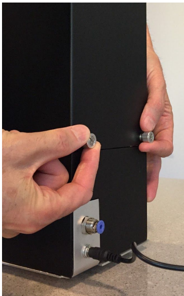
(Fig-1) Cover removal
